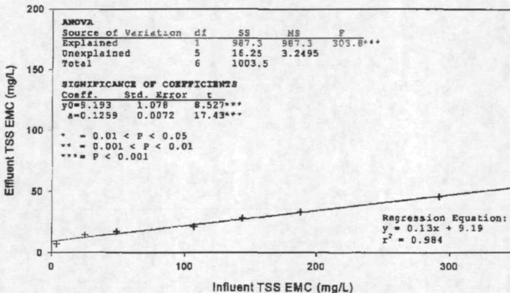
Figure 3. Regression analysis applied to the TSS data associated with the estimation of the SCS 106 TSS removal efficiency of the ZPG™ StormFilter cartridge at 28 L/min. The solid line is the regression. The dotted lines signify the lower and upper 95% confidence intervals. ANOVA indicates a significant (P<0.001) linear relationship between influent and effluent TSS EMC.
