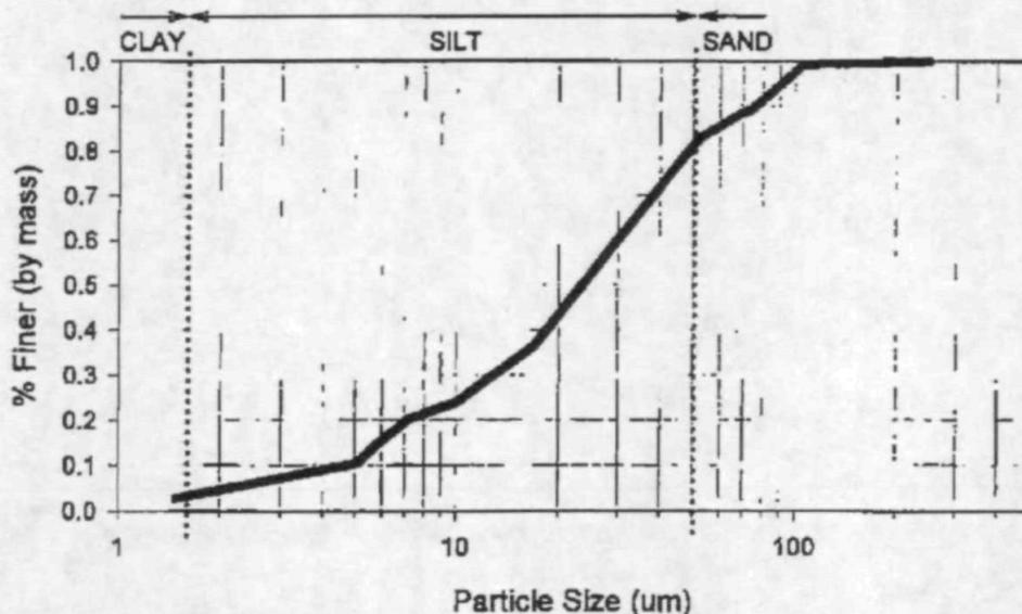
Figure 1. Particle size distribution for SCS 106. Sand/silt/clay fractions according to USDA definitions are approximately 20%, 80%, and 0% for SCS 106, indicating that the texture corresponds to a silt material.
