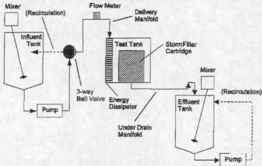
Figure 2. Schematic diagram of the cartridge-scale test apparatus. Arrows indicate flow pathways. Dashed arrows indicate recirculation pathways employed during influent and effluent sampling.
