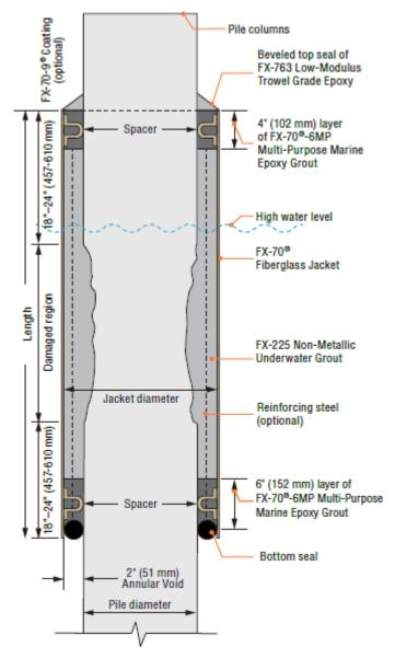
Figure 3 – Section of Simpson Strong Tie Jacket in Place (Source: Simpson Strong-Tie, Material Specs)
