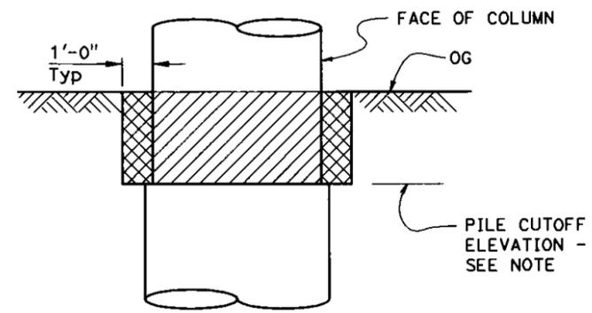
NOTE: For specified pile cut-off elevation, see "PILE DATA TABLE" this sheet
