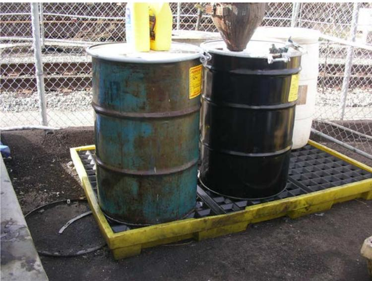
Photo 11. Hazardous waste drums on secondary containment. There was water in the secondary containment. A worker was adding material to the drum on the right with the funnel.
