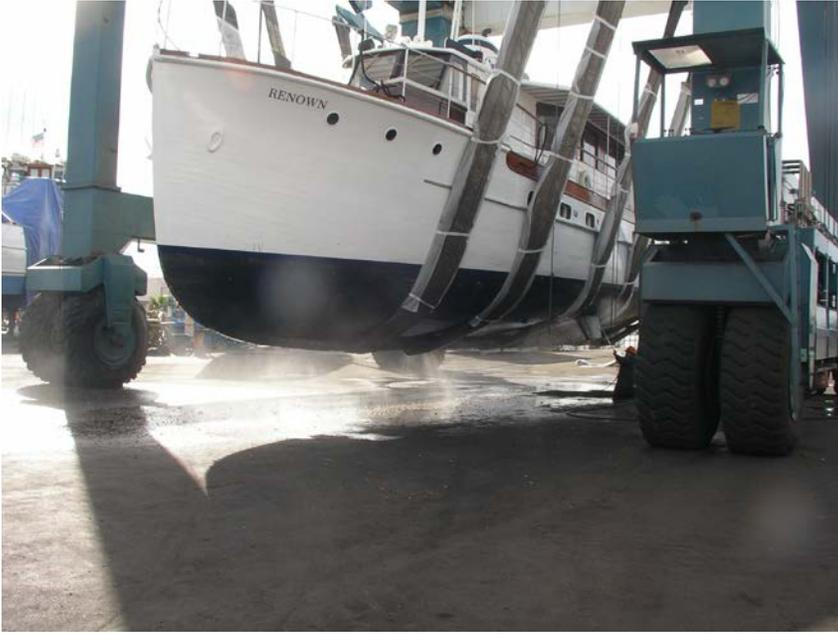
Photo 13. Boat being washed near travel lift pier. Water flowed into a catch basin. A pump could be heard pumping water to the 50,000 gallon tank.
