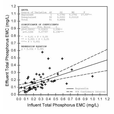
**Figure 1.** <u>Sand filter</u> data analyzed using Regression of EMC for Total Phosphorus (TP) removal representing 52 paired influent and effluent samples at 5 roadway sites and demonstrating a mean removal efficiency estimate of 67% with 95% confidence intervals of 52% and 83%. Data was statistically significant at the P <0.001 level.
