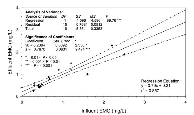
Figure 2. Nitrate Nitrogen (NO<sub>3</sub> -N) EMC data for the KMMS StormFilter system with coarse perlite/coarse zeolite cartridges with a design flow rate of 15 gpm/cartridge. Using the regression of EMC performance evaluation method, NO<sub>3</sub> -N removal is estimated to be 21% (P=0.05: L1=39%, L2=4%).
