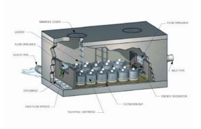
*Figure 1:* The Pre-cast 2.5 x 7 m StormFilter
