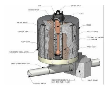
Figure 2: The StormFilter cartridge
