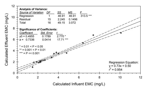
Figure 3. Total nitrogen EMC data extrapolated from available TK-N and  $NO_3$ -N data for the KMMS StormFilter system with coarse perlite/coarse zeolite cartridges with a design flow rate of 15 gpm/cartridge. Using the regression of EMC performance evaluation method, total nitrogen removal is estimated to be 27% (P=0.05: L1=35%, L2=18%).
