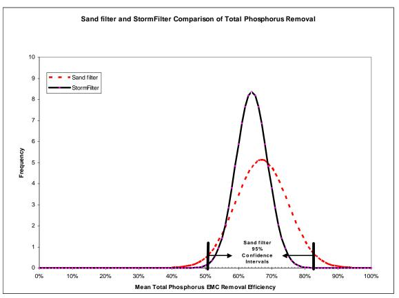
**Figure 3.** A comparative analysis of the StormFilter and sand filter data that displays the probability distribution of the mean total phosphorus removal performance of these two types of media filters. A total of 9 sites, each data set containing over 50 storm events were used in the comparison. The overlap of the two bell shaped curves indicate that there is no statistical difference between the performance of the StormFilter and sand filters for the removal of total phosphorus.
