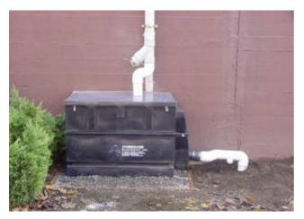
The objective of the test was to evaluate both the removal effectiveness and the longevity of the filter. A total of 10 discrete samples show a mean removal rate of 43%, while data for copper show a mean removal rate of 92%
