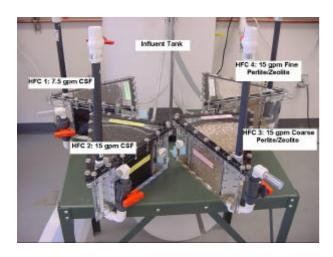
The samples were then transported to the wet lab, continuously stirred with a mixer and run through a series of horizontal flow columns shown in Photo 3.
