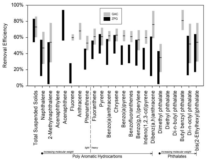
Figure 2. Graphical comparison of ZPG and GAC treatment performance. Absent bars indicate a regression that was not significant at the 95% confidence level or better.
