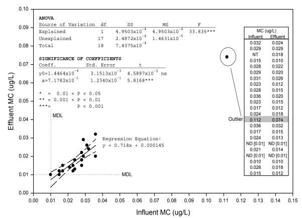
Figure 1. An example of regression analysis of the 2-Methylnaphthalene results for the ZPG data including the ANOVA table used to assess the significance of the regression and the error statistics of regression coefficients. Note that the indicated outlier is not included in the regression analysis (see Results and Discussion section). MDL = Method Detection Limit.
