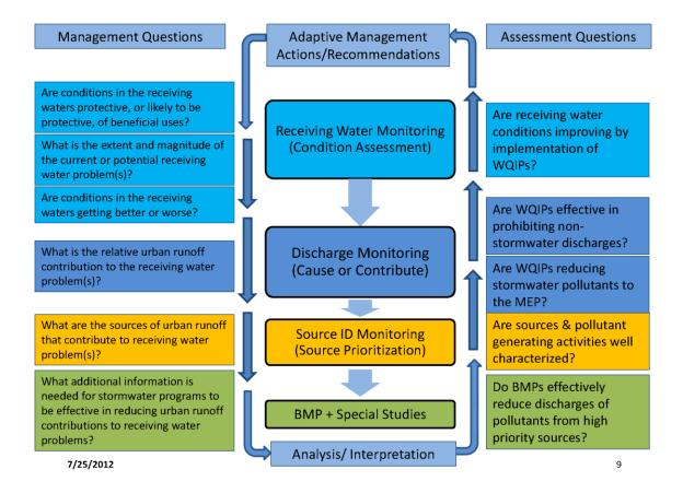
The administrative draft permit focuses on the top four management questions, the receiving water and discharge monitoring, and assessment. There are two more levels needed: source identification and special studies/BMPs. The top three (blue) deal with receiving waters. The next one (darker blue) is discharge monitoring. Yellow is source identification and pollutant-generating activity (PGA) monitoring and identification. The bottom (green) is special studies.
