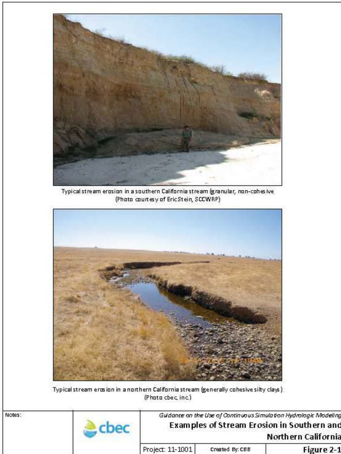
Figure 2-1. a. Example of a loosely consolidated, non-cohesive sand and gravel stream bed. b. Example of a relatively cohesive silty-clay stream bed.
