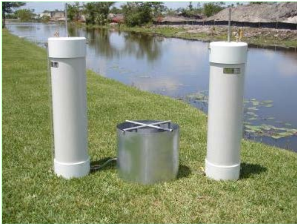
Photo 4- Double Ring Infiltrometer Set-up with Mariotte Tubes (Photo courtesy of Turf-Tec International)
