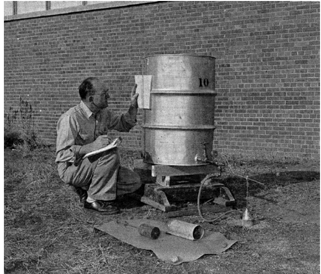
Photo 7 - Typical Well Permeameter Test Installation
