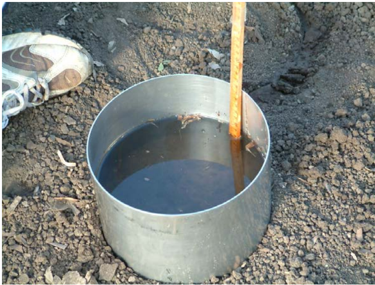
Photo 1 – Simple Single Ring Infiltrometer
