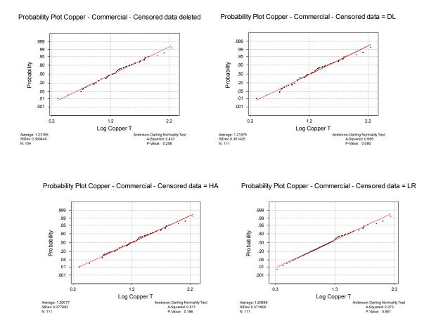
Figure C1. Probability plot for different replacements of the censored data for copper
