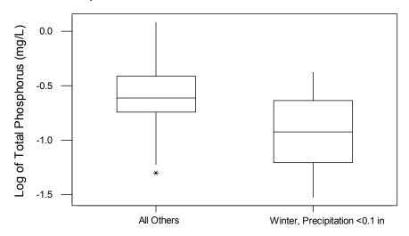
Figure 66. Box and whiskers plot for residential total phosphorus concentrations for sites having > 27% impervious surfaces
