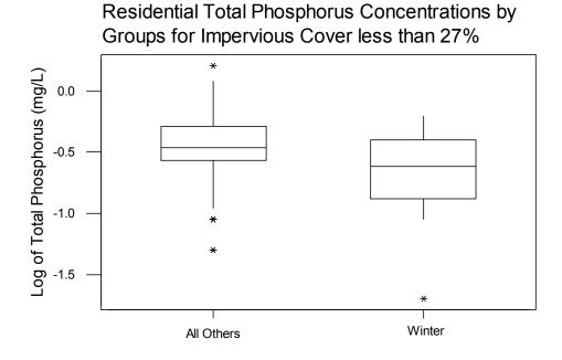
Figure 64. Box and whiskers plot for residential total phosphorus concentrations for sites having < 27% impervious surfaces
