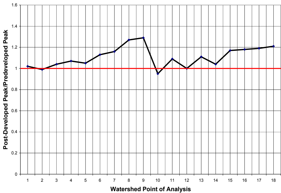
Figure 10-5: Comparison of 100-Year Pre- and Post-Developed Peak Rates with Peak Rate Controls, Devils Brook Watershed
