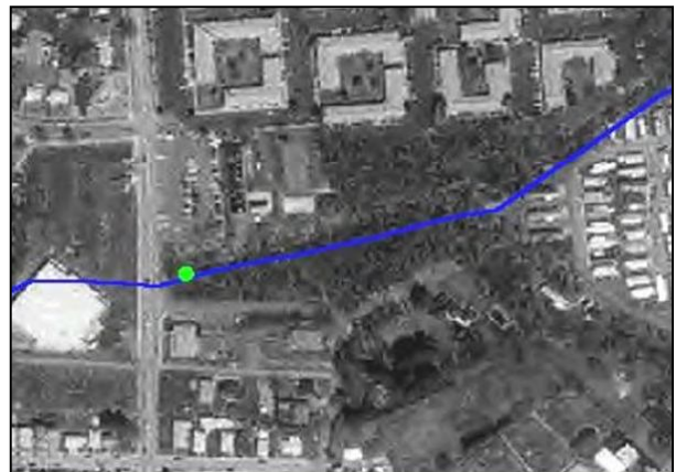
Figure 4: Crossing retrofits are easy to find when road network and drainage layers are superimposed.
