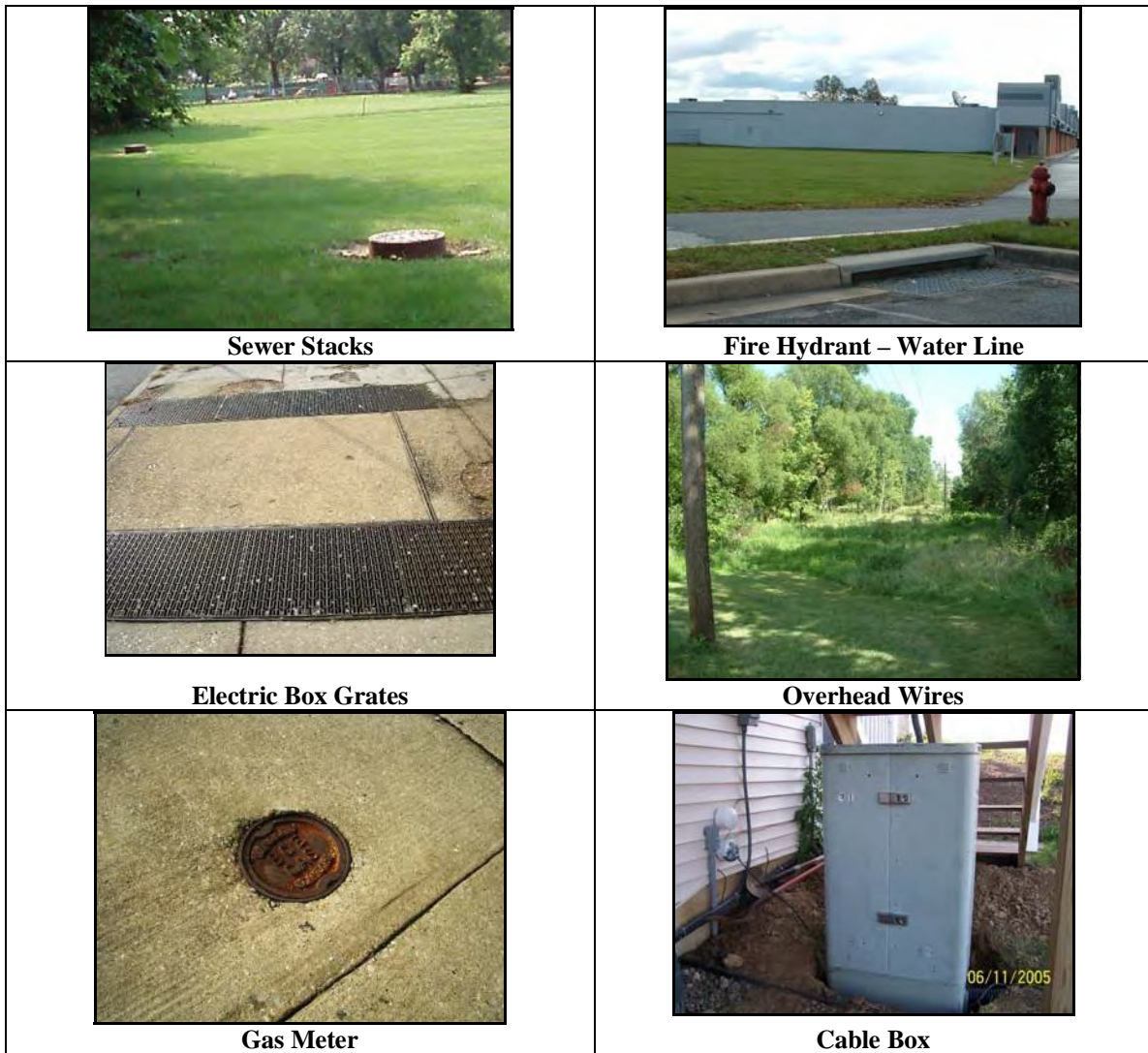
Figure 4.11: Examples of Some Common Utility Indicators
