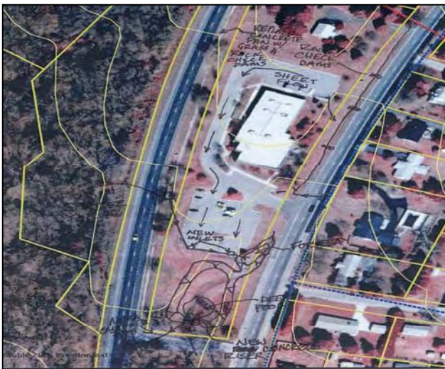
Figure 6: Orthophotos can help find small parking lots and for concept sketches.
