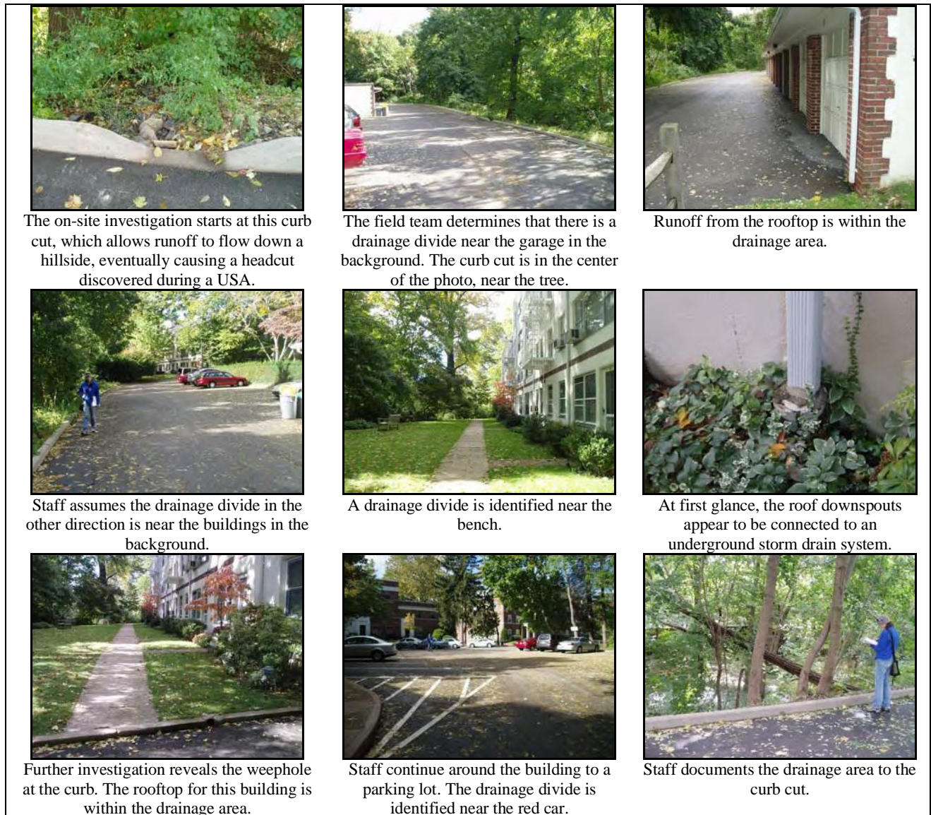
Figure 4.6: Investigating the drainage area at an apartment complex
