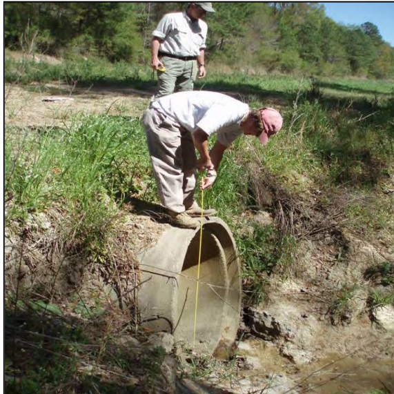
Figure 7: Crews measure the diameter, condition and invert elevation of the storm drain outfall.
