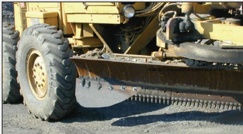
Figure 4.18—Homemade ditch cleaner for a grader.
