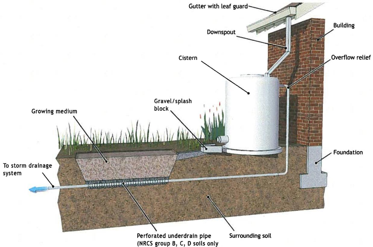
Figure 7. Cistern with Bioretention BMP Example Illustration
