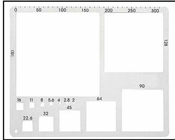
(b) US SAH-97 half-phi template (gravelometer) NOT to scale
