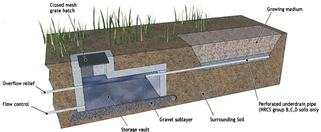
**Figure 8. Bioretention with Vault BMP Example Illustration**
