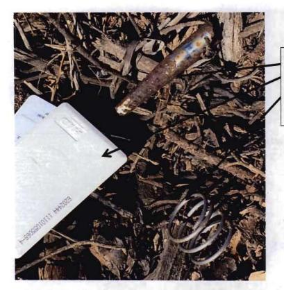
Contaminants observed in mulch applied for erosion control on side slopes. Water Board staff access card show for size comparison.
