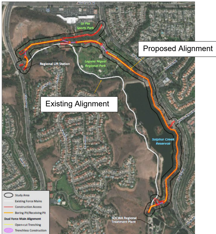
Figure 3. Regional Lift Station Force Main Replacement Project; Existing and Proposed Sewer Alignments 15
