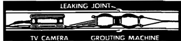
When a leak is located by the TV camera, our technician stationed in a mobile laboratory at the job-site can isolate and seal the leak, usually in less than a minute.
