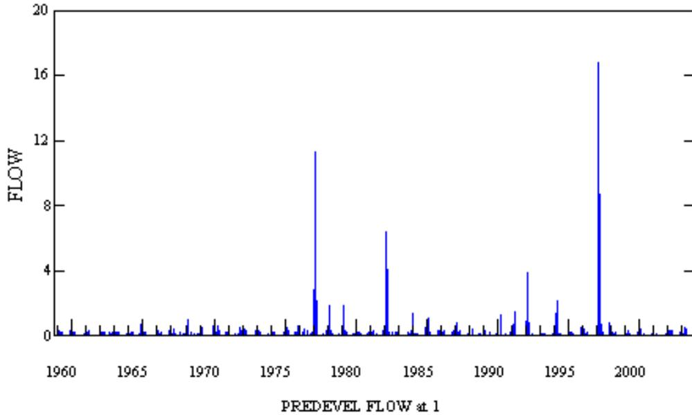
Figure 6-8. Pre-Developed Flow Time Series for Basin A
