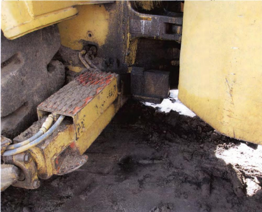
Photo 29: More spills or leaks from construction vehicle.
