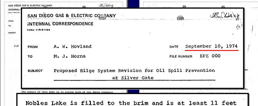
Nobles Lake is filled to the brim and is at least 11 feet deep with a mixture of oil and earth. It is no longer an acceptable settling pond. It is not desirable to pump any additional bilge water to it.
