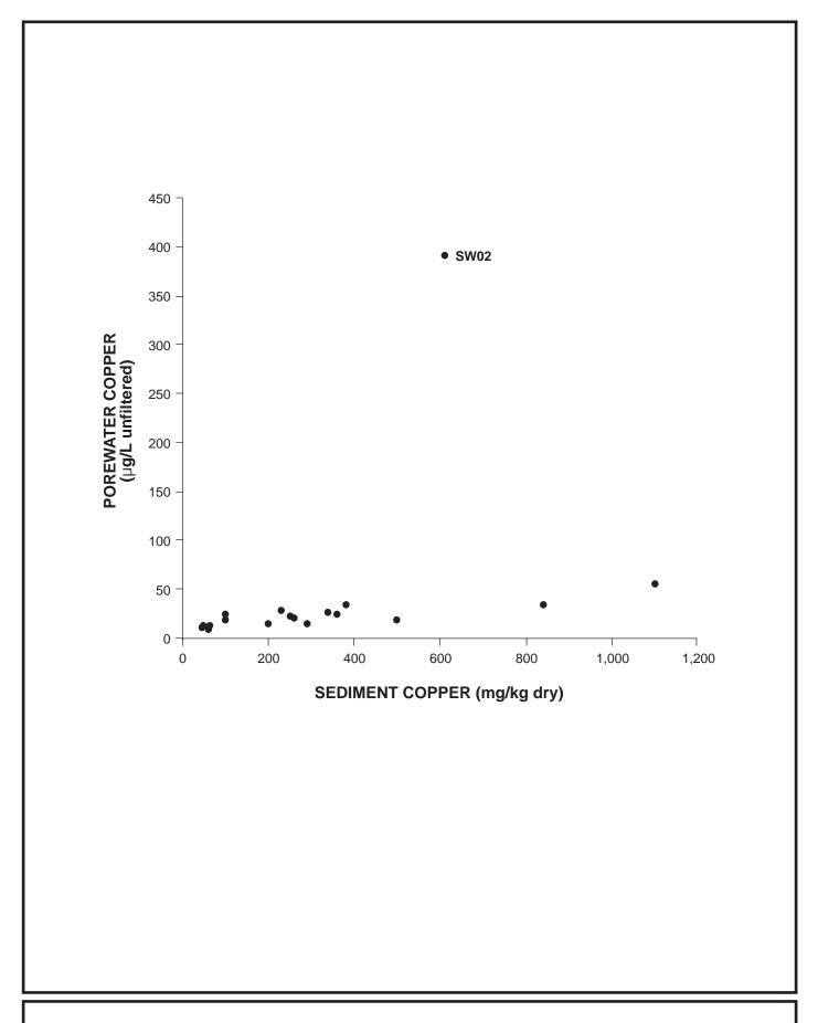
Figure 4-23. Copper concentrations in sediment and associated pore water
