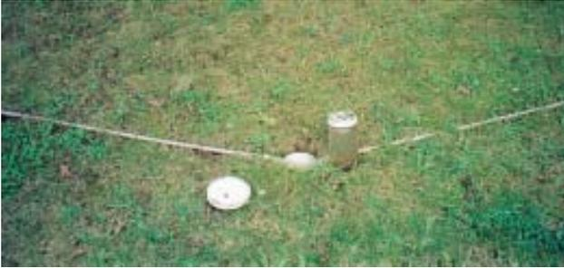
Figure 3. Tube-type lawn sampler (site 2).
