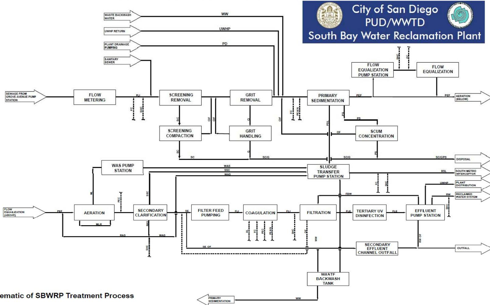
**Schematic of SBWRP Treatment Process**
