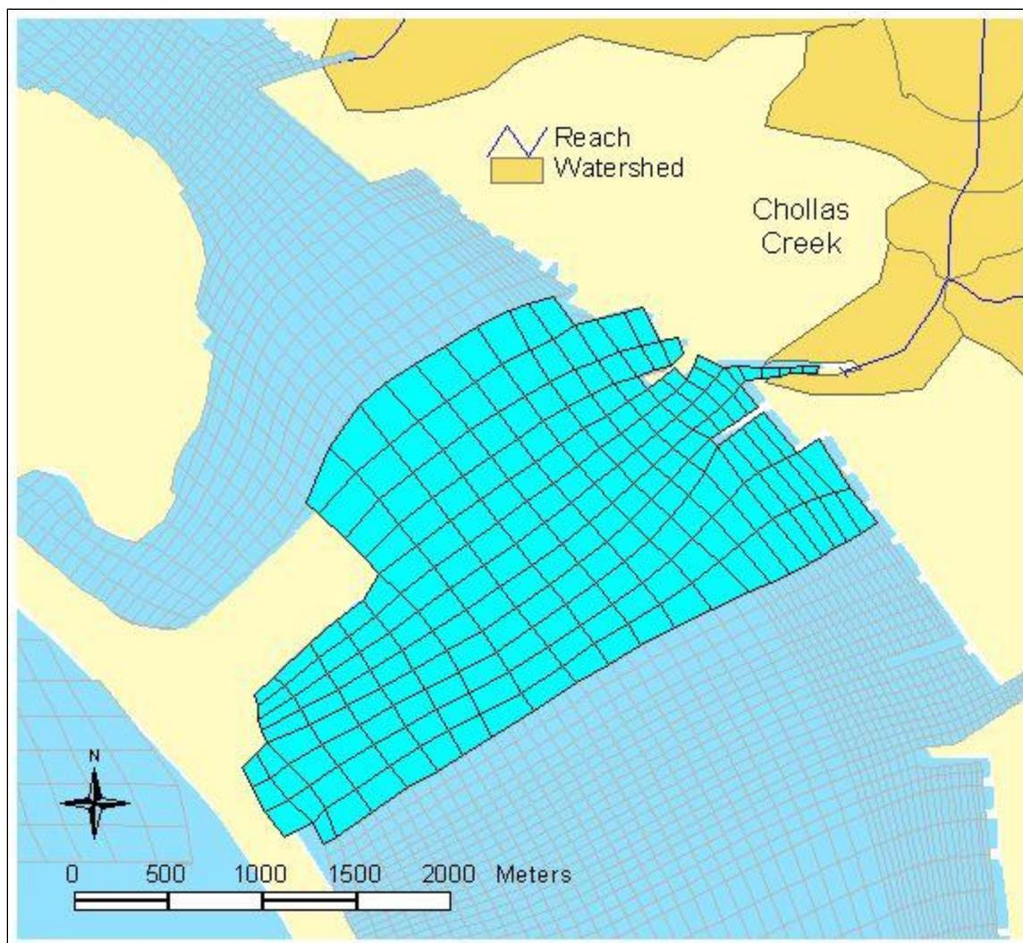
**Figure 6.2. EFDC grid for the sediment transport and toxics model for the mouth of Chollas Creek.**
