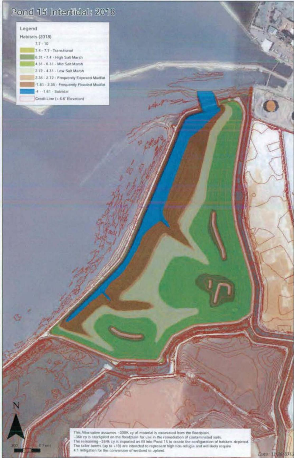
This Alternative assumes ~300k cy of material is excavated from the floodplain, ~36k cy is stockpiled on the floodplain for use in the remediation of contaminated soils. The remaining ~264k cy is imported as fill into Pond 15 to create the configuration of habitats depicted. The taller berms (up to +10) are intended to represent high tide refugia and will likely require 4:1 mitigation for the conversion of wetland to upland.
