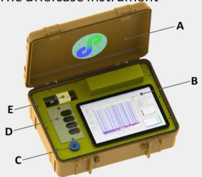
A) The portable brief-case format with external power & recharge outlet, B) The tablet PC with control and data analysis GUI, C) The sample injection port, D) The rapid-replace consumable reagent bay, and E) The target primer library.
