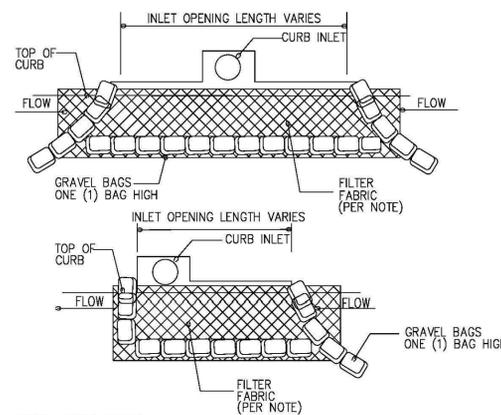
STORM DRAIN INLET PROTECTION
