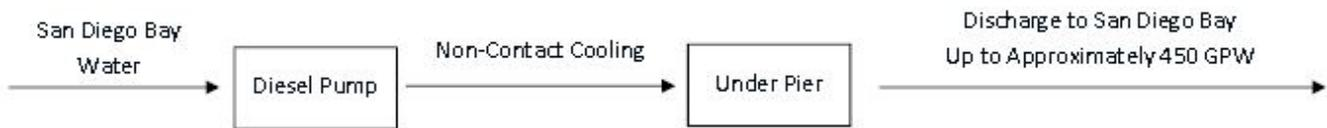
**Figure C-3. Utility Vault and Manhole Dewatering Discharges**
