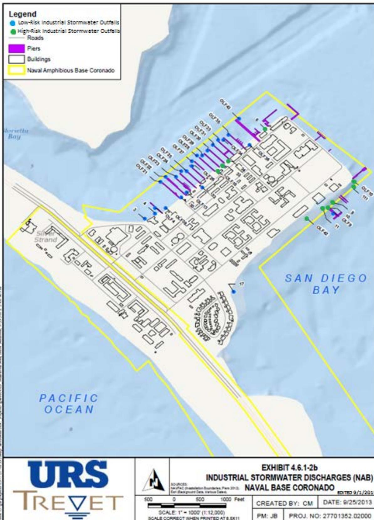
Figure B-12. NBC Industrial Stormwater Discharge Locations at NOLF
