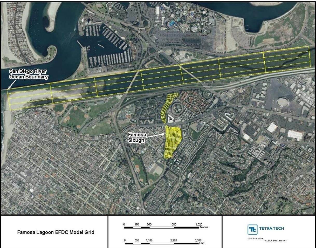
Figure 47. EFDC Grid for Slough, Channel, and the San Diego River
