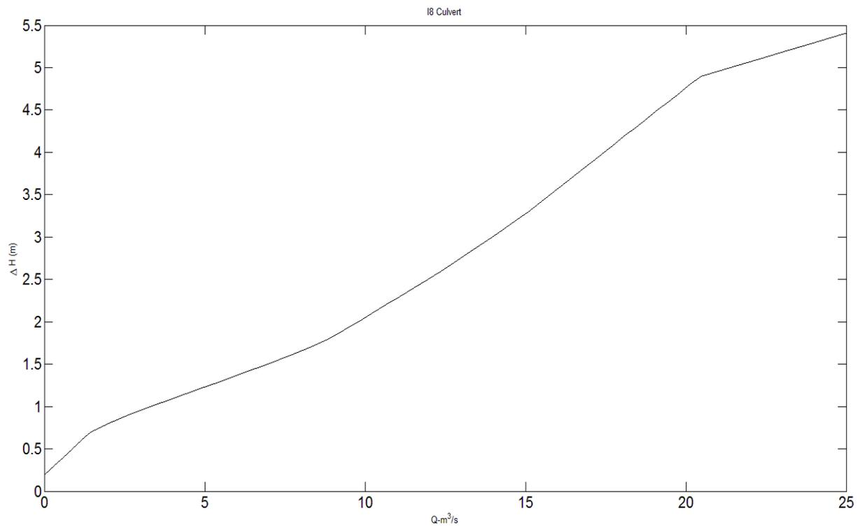
Figure 48. Flow Control Plot for the RC Culverts under I-8
