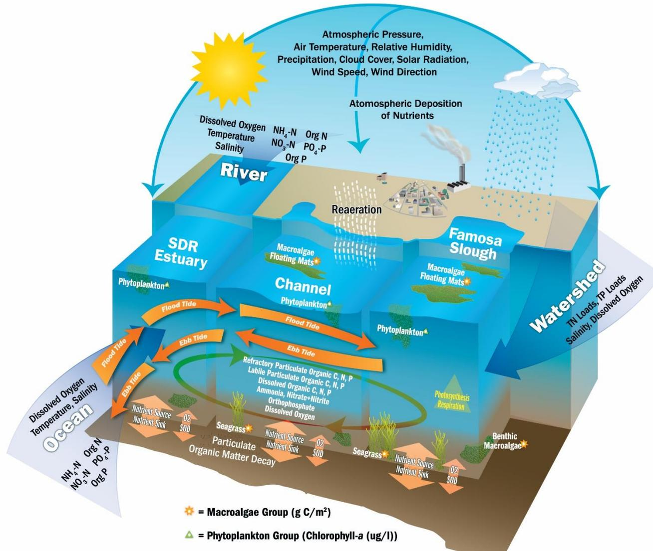
Figure 52. Schematic Diagram of Famosa Slough Receiving Water Model Processes
