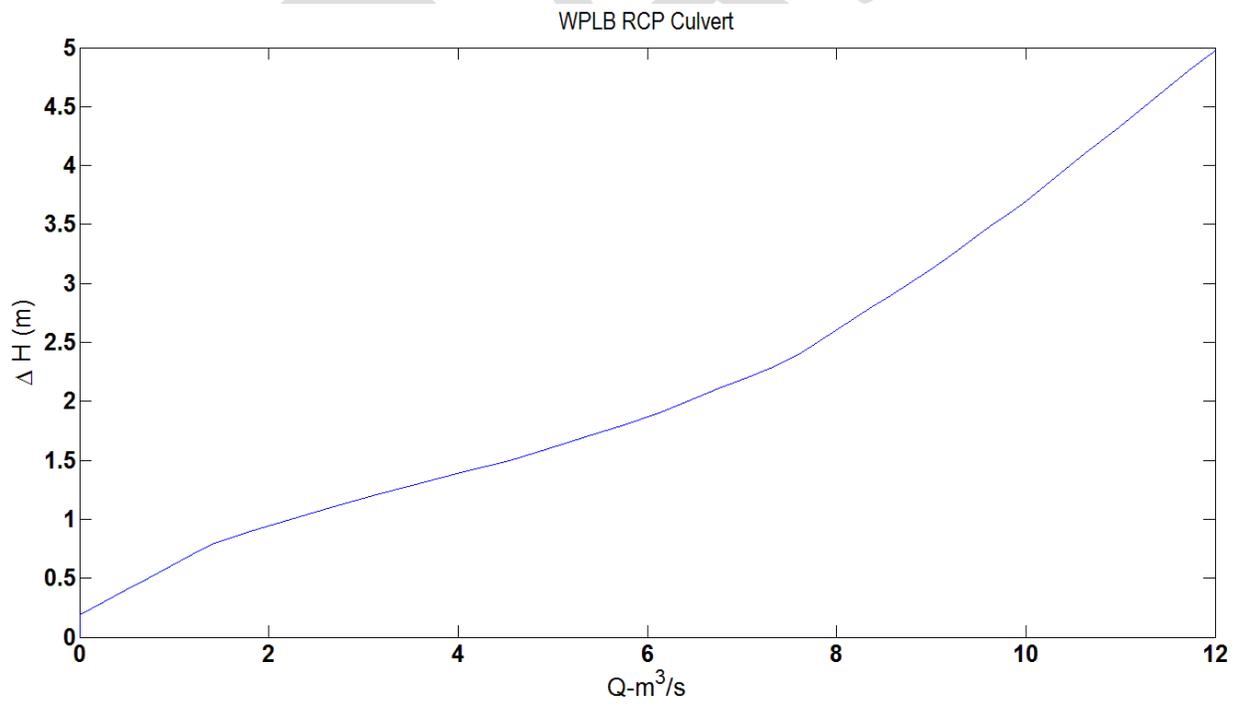
Figure 49. Flow Control Plot for the RC Culverts at WPLB
