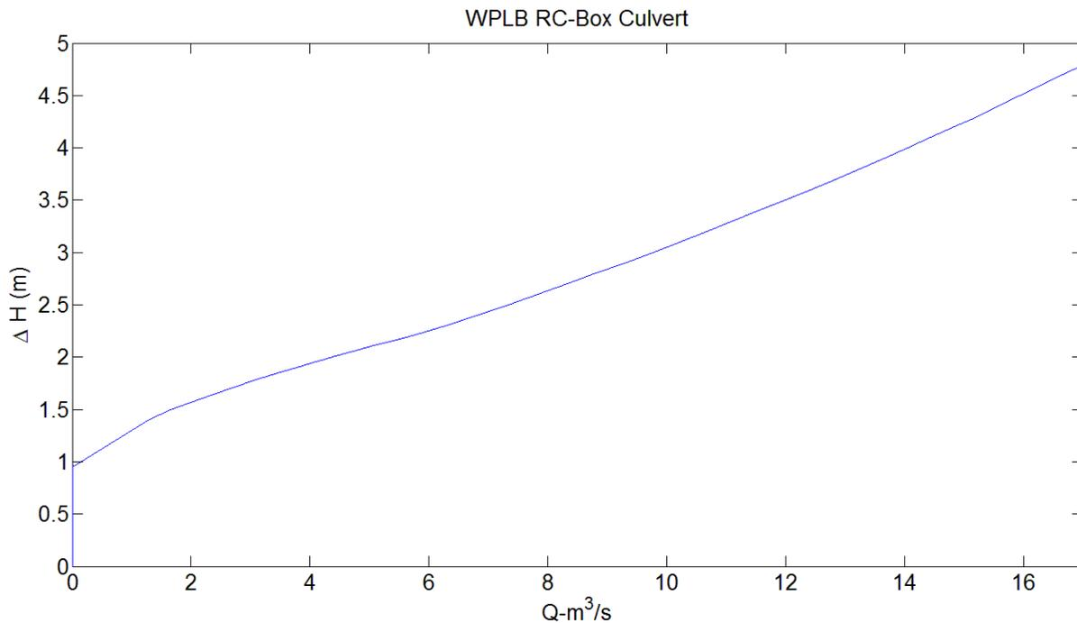
Figure 50. Flow Control Plot for the RC Box Culvert at WPLB
