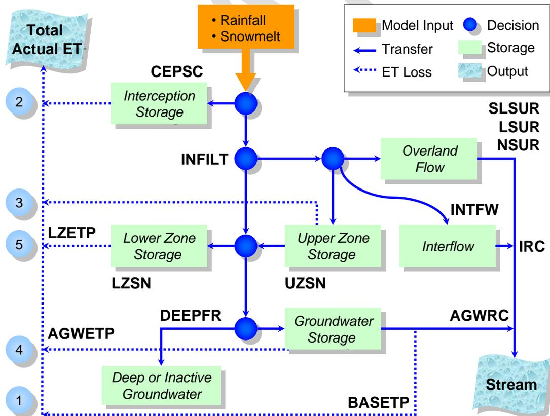
Figure 2. Schematic of LSPC Hydrology Components
