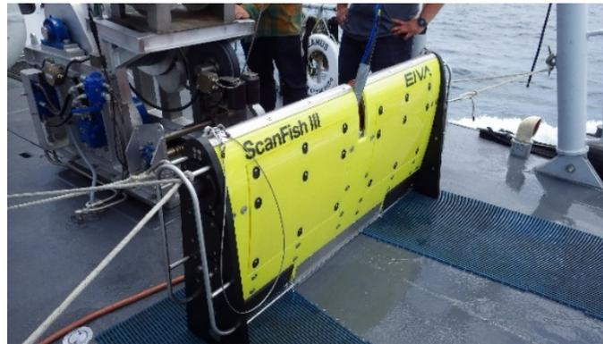
Remotely Operated Towed Vehicle (ROTV)
