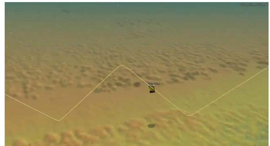
Simulation of ROTV movement throughout water column.
