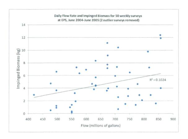
Whereas Encina's average intake flow during the 2004/2005 sampling period was 632.6 MGD, <sup>46</sup> the Project's maximum intake flow will be only 304 MGD. Because the Project's flow volumes will be less than Encina's, its impingement impacts are also proportionally less than the Project's projected impacts.
