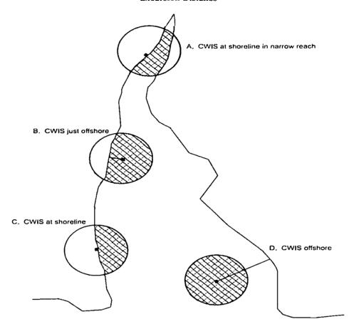
CWIS = Cooling Water Intake Structure
