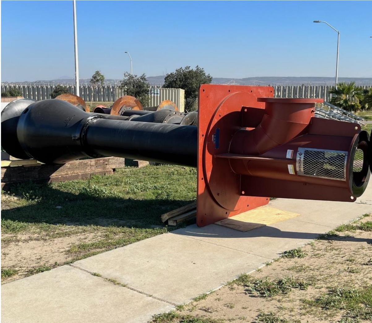
*Figure 6: Closer view of one of the two new influent pumps. (USIBWC 12/13/2023)*
