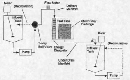
Figure 2. Schematic diagram of the cartridge-scale test apparatus. Arrows indicate flow pathways. Dashed arrows indicate recirculation pathways employed during influent and effluent sampling.
