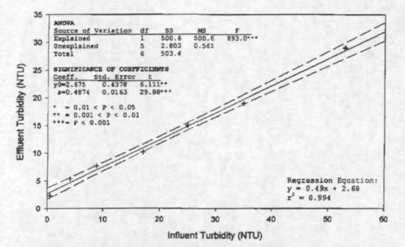
Figure 4. SCS 106 turbidity reduction by the ZPG™ StormFilter cartridge at 28 L/min. The solid line is the regression. The dotted lines signify the upper and lower 95% confidence intervals. ANOVA indicates a significant (P<0.001) linear relationship between influent and effluent turbidity.
