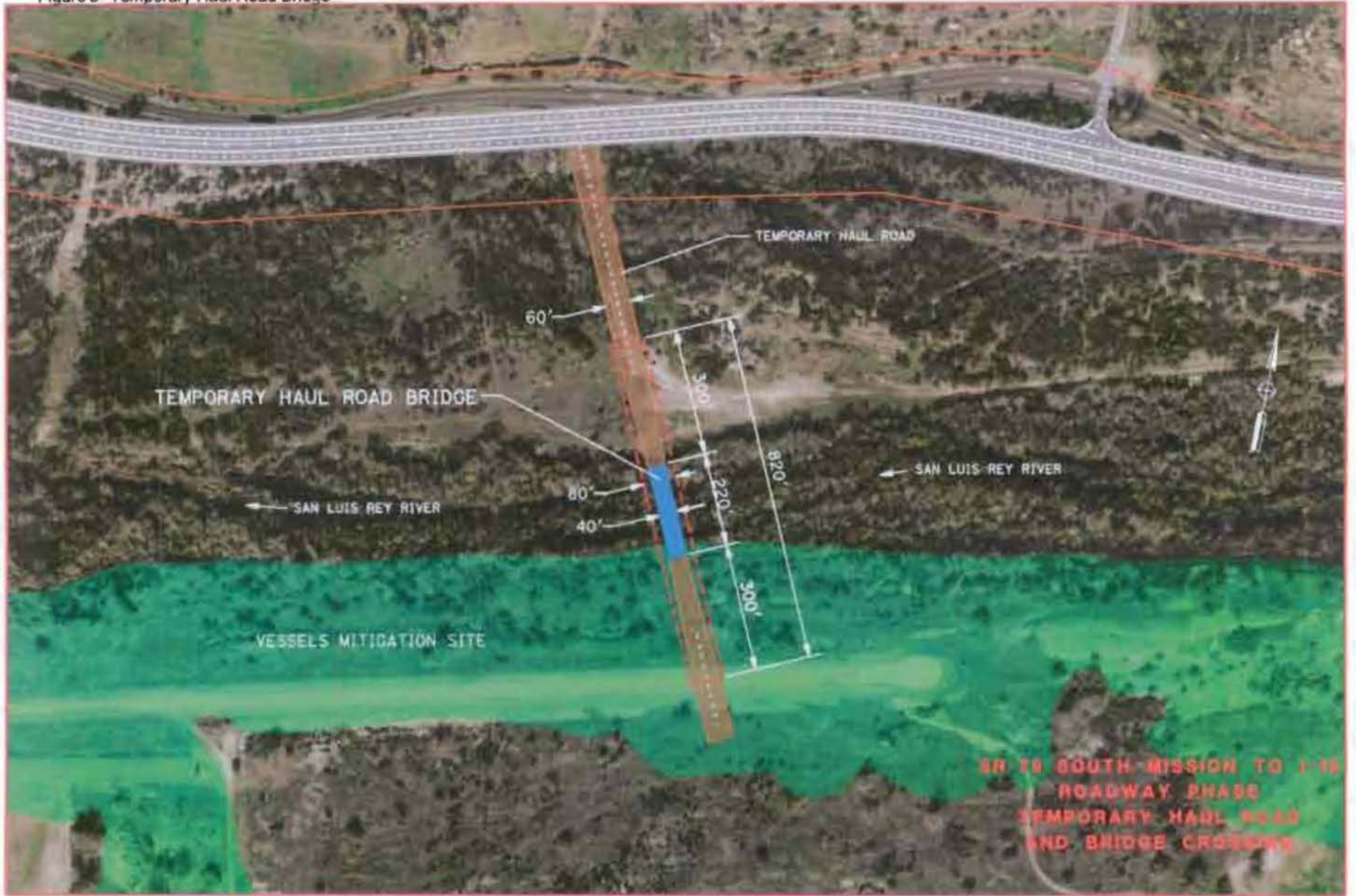
Figure 5 Temporary Haul Road Bridge
