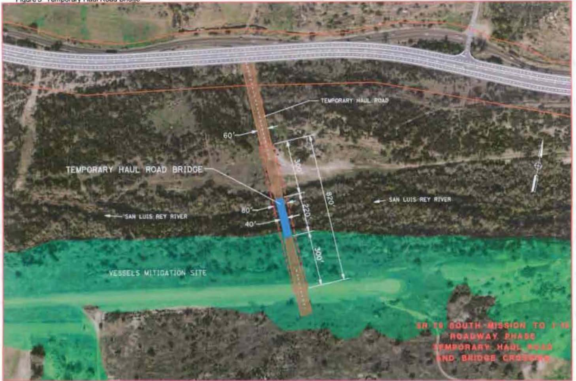
Figure 5 Temporary Haul Road Bridge
