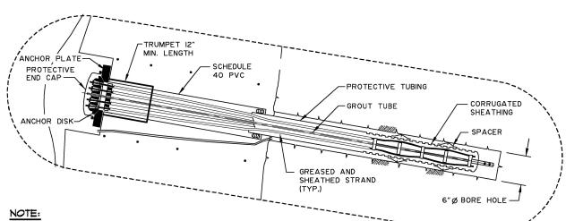
ANCHOR PLATE, TRUMPET & PROTECTIVE END CAP SHALL BE HOT DIP GALVANIZED
