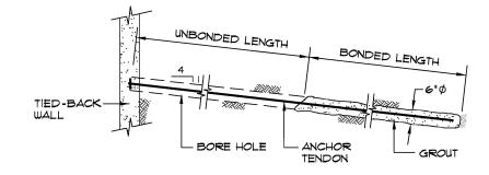
TYPICAL ANCHOR SCHEMATIC
