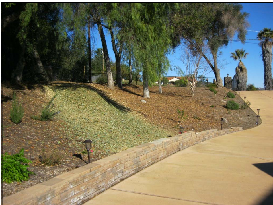
Below Photo: The exposed and vulnerable area has been mulched with wood chips and compost and planted with native, low-water use plants to help prevent and control sediment loss. The high-water use lawn has been replaced with mulch and low water use plants as well. The BMPs implemented were mulching and critical area planting. Photo taken during the follow-up site visit.
