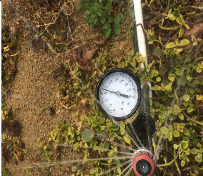
Photo 1: Dynamic irrigation pressure reading of 72 psi.
