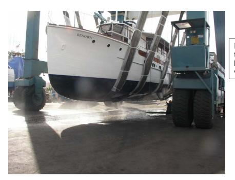
Photo 13. Boat being washed near travel lift pier. Water flowed into a catch basin. A pump could be heard pumping water to the 50,000 gallon tank.
