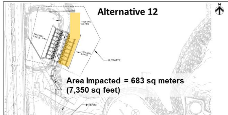
**Note that the design has expanded from 8 to 16 screens to ensure that no velocity upstream of the screen face is above 0.5 ft/sec**
