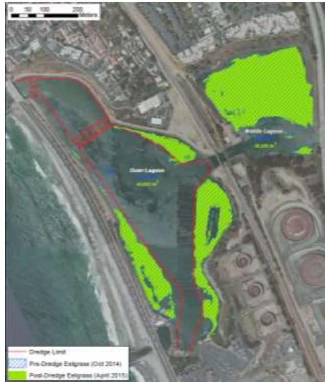
**Figure 16. 2015 post-dredge eelgrass survey in Outer Lagoon of Agua Hedionda Lagoon (image from Merkel and Associates 2015).**
