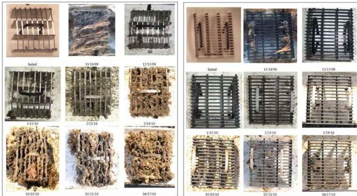
Figure 4.5-2. Biofouling of duplex coupon (#1) from November 16, 2009 to June 17, 2010.
