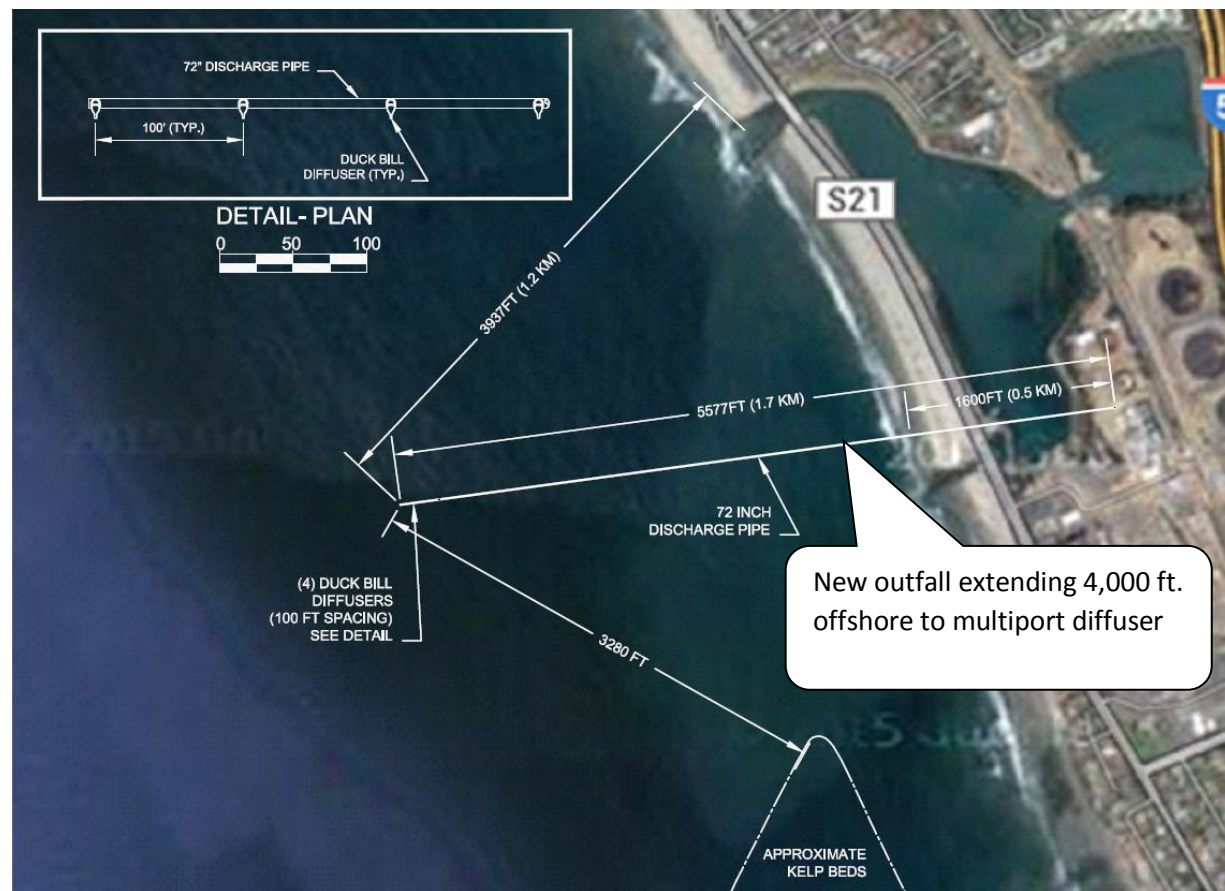
Figure 9. General schematic of new outfall extending 4,000 feet offshore to a multiport diffuser.
