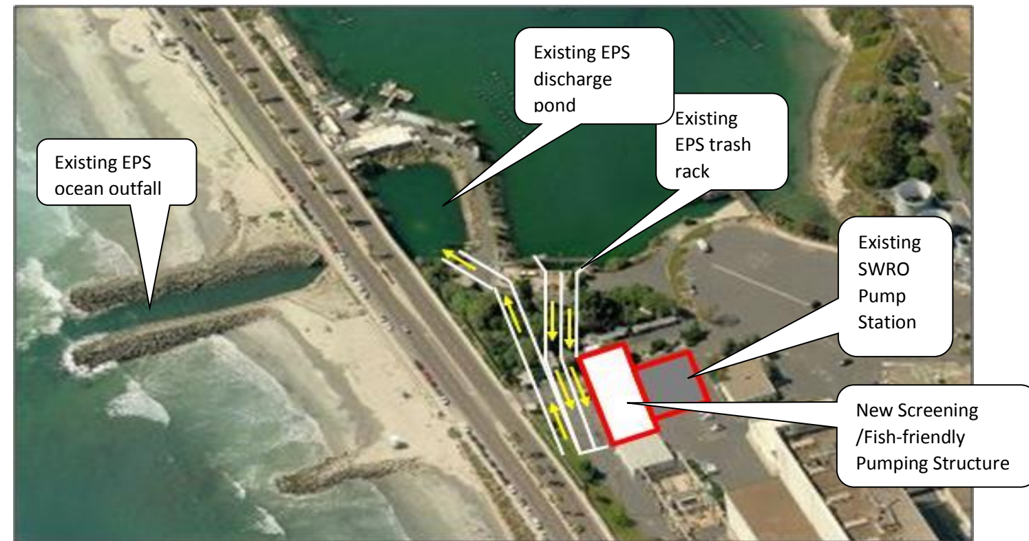
Figure 4. General schematic of the layout of the Expanded CDP with a screened intake and discharge flow augmentation.
