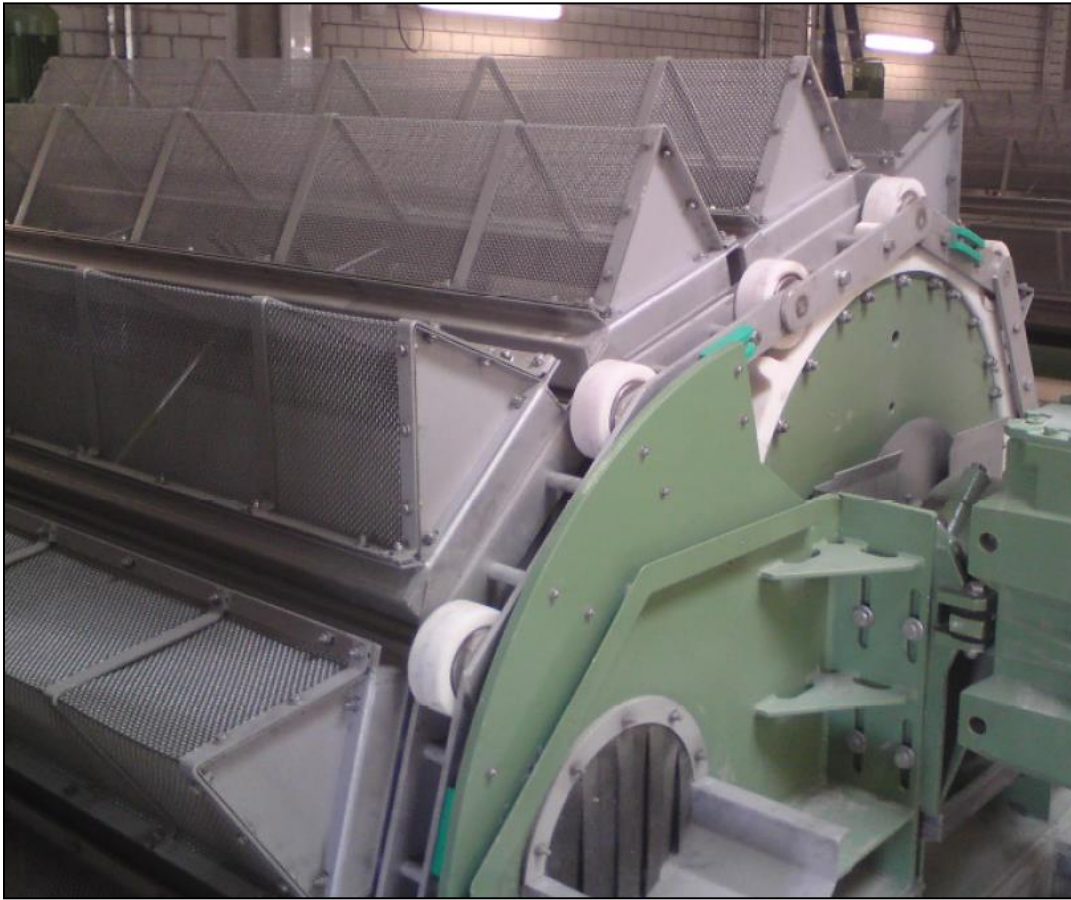
Figure 28. Example of BWT center-flow traveling screen panel mesh (courtesy Bilfinger Water Technologies).
