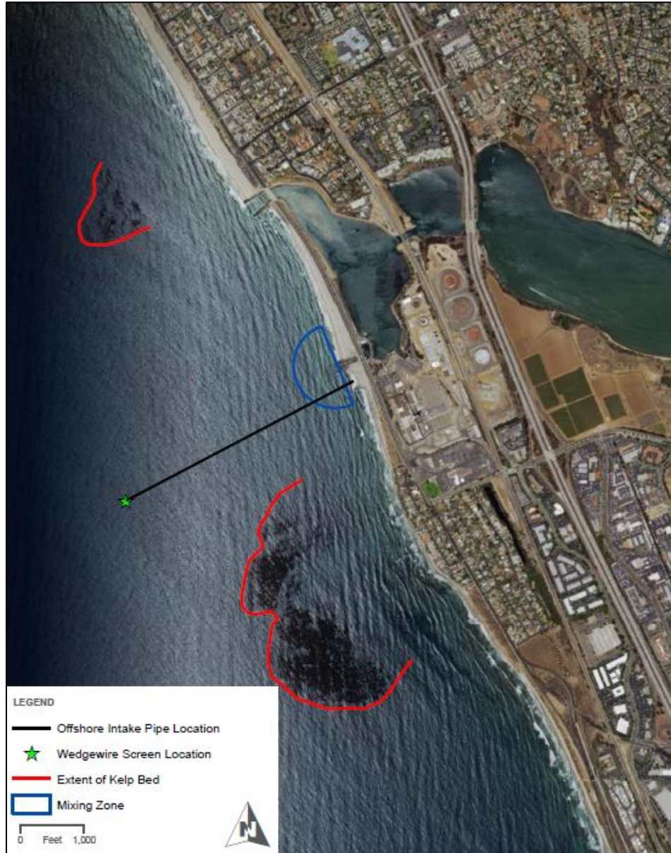
Figure 2. Location of wedgewire screen array relative to existing kelp beds and brine mixing zone. Location of kelp beds was estimated based on Google Earth aerial and MBC 2013.
