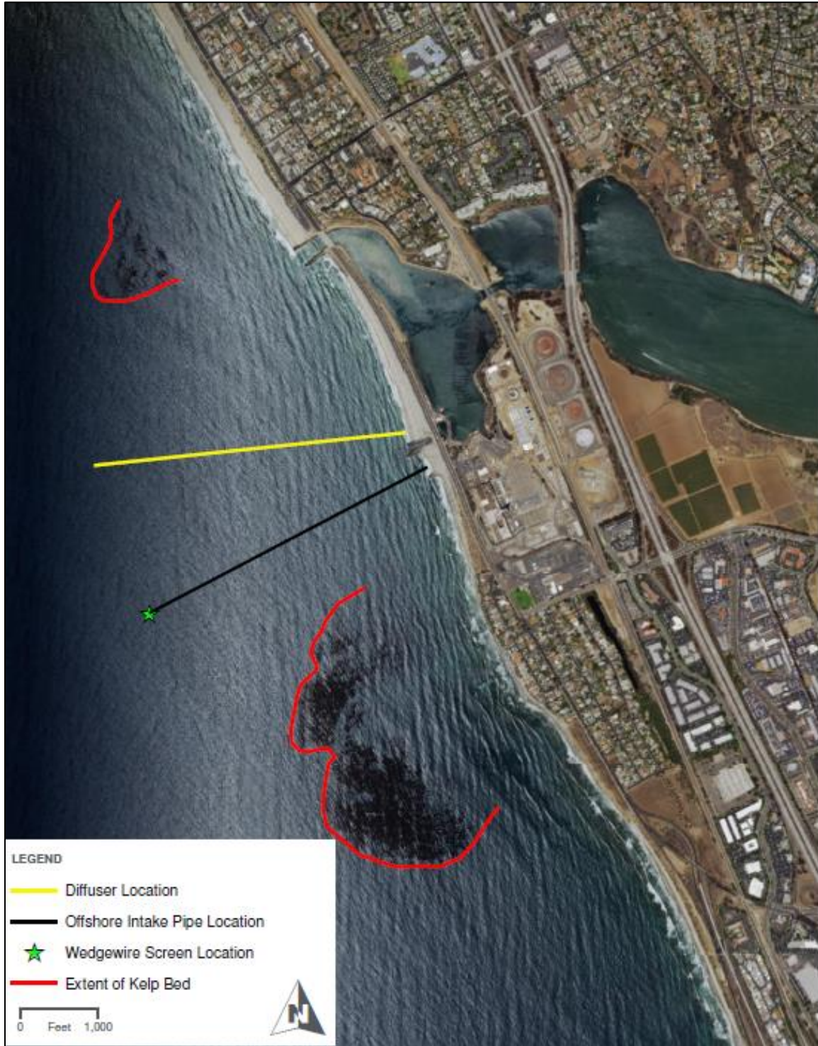
Figure 10. Location of wedgewire screen array relative to existing kelp beds. Location of kelp beds was estimated based on Google Earth aerial and MBC 2013.
