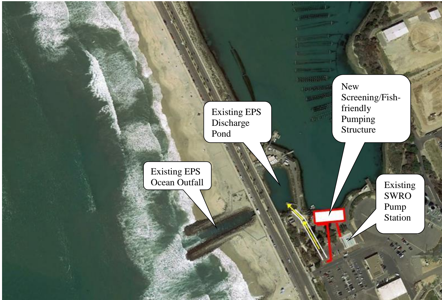
Figure 22. General schematic of the CDP with Lagoon-based Shoreline 1-mm traveling water screens and flow augmentation.
