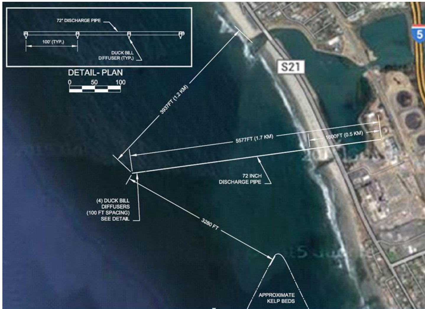
Figure 9. General schematic of the layout of the CDP discharge diffuser array. Note the WWS array has been omitted from the drawing for clarity.
