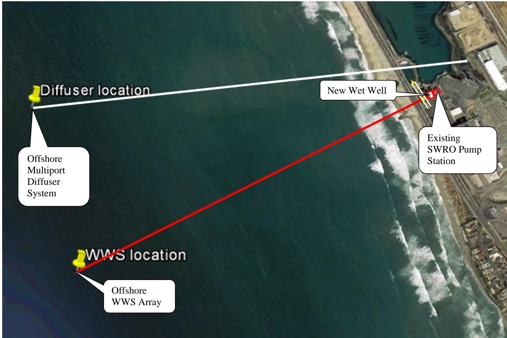
Figure 8. General schematic of the layout of the CDP with an offshore screened intake and discharge diffuser.
