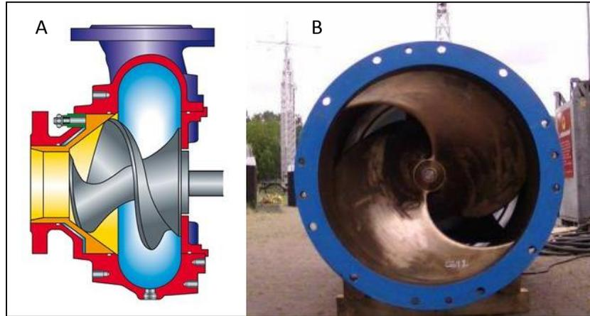
Figure 3. (A) Cut away diagram of a screw centrifugal impeller (Source: Hidrostal) and (B) impeller of Bedford pumps SAF.90.05.12 (Source: Spierts and Vis 2012).
