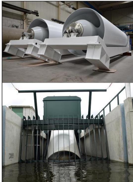
Figure 1. Screw pumps mounted in diagonal pipes (Source: Fish Flow Innovations).
