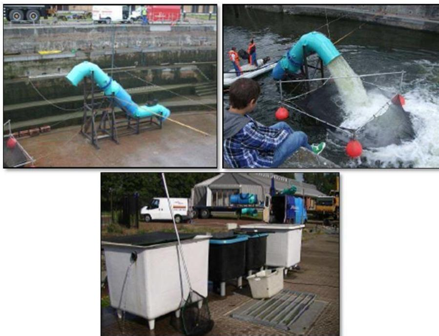
**Figure 5. Photos of the pump passage test facility in the Netherlands. Clockwise from top left: pump test facility, discharge of pump into net pen during testing, and latent mortality holding tanks.**
