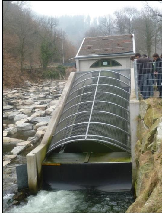
Figure 2. Screw pump mounted in open trough in a hydropower application (<https://parlonsenergie.wordpress.com/tag/fribourg/>).
