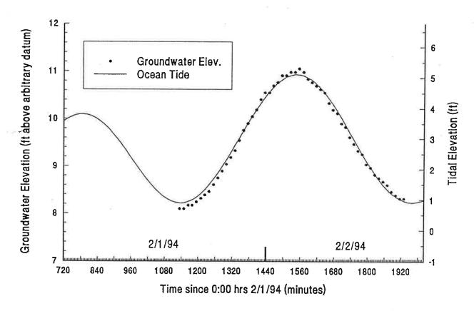
TIDAL DATA HAS BEEN SHIFTED TO ACCOUNT FOR A 25-MINUTE TIME LAG BETWEEN PREDICTED TIDAL PEAKS AT SCRIPPS PIER AND THE OBSERVED PEAKS IN PRODUCTION WELL W-1
