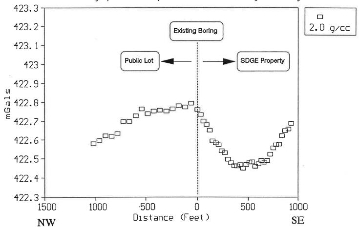
Figure #1 - Relative gravity profile calculated for a bulk density of 2.0 g/cc.
