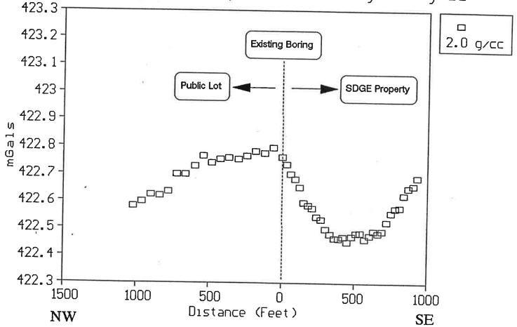
Figure #1 - Relative gravity profile calculated for a bulk density of 2.0 g/cc. Data has been corrected for elevation, drift, and nearby terrain.
