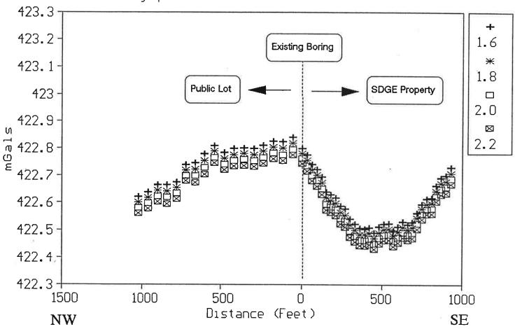
Figure #2 - Relative gravity profile calculated for a bulk density range from 1.6 g/cc to 2.2 g/cc. data has been corrected for elevation, drift, and nearby terrain.
