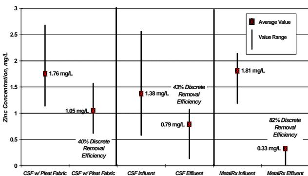
*Figure 2 – Metals Removal*
