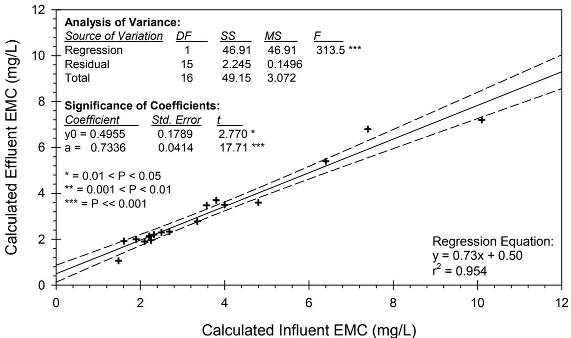
Figure 3. Total nitrogen EMC data extrapolated from available TK-N and NO<sub>3</sub><sup>-</sup>-N data for the KMMS StormFilter system with coarse perlite/coarse zeolite cartridges with a design flow rate of 15 gpm/cartridge. Using the regression of EMC performance evaluation method, total nitrogen removal is estimated to be 27% (P=0.05: L1=35%, L2=18%).
