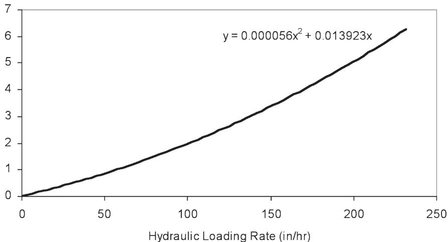
**Figure 2: Hydraulic Loading Characteristics of the UrbanGreen BioFilter**
