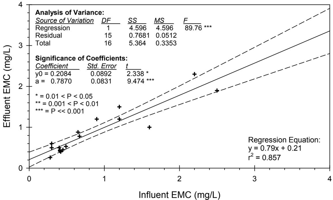
Figure 2. Nitrate Nitrogen (NO<sub>3</sub><sup>-</sup>-N) EMC data for the KMMS StormFilter system with coarse perlite/coarse zeolite cartridges with a design flow rate of 15 gpm/cartridge. Using the regression of EMC performance evaluation method, NO<sub>3</sub><sup>-</sup>-N removal is estimated to be 21% (P=0.05: L1=39%, L2=4%).
