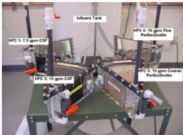
The samples were then transported to the wet lab, continuously stirred with a mixer and run through a series of horizontal flow columns shown in Photo 3.
