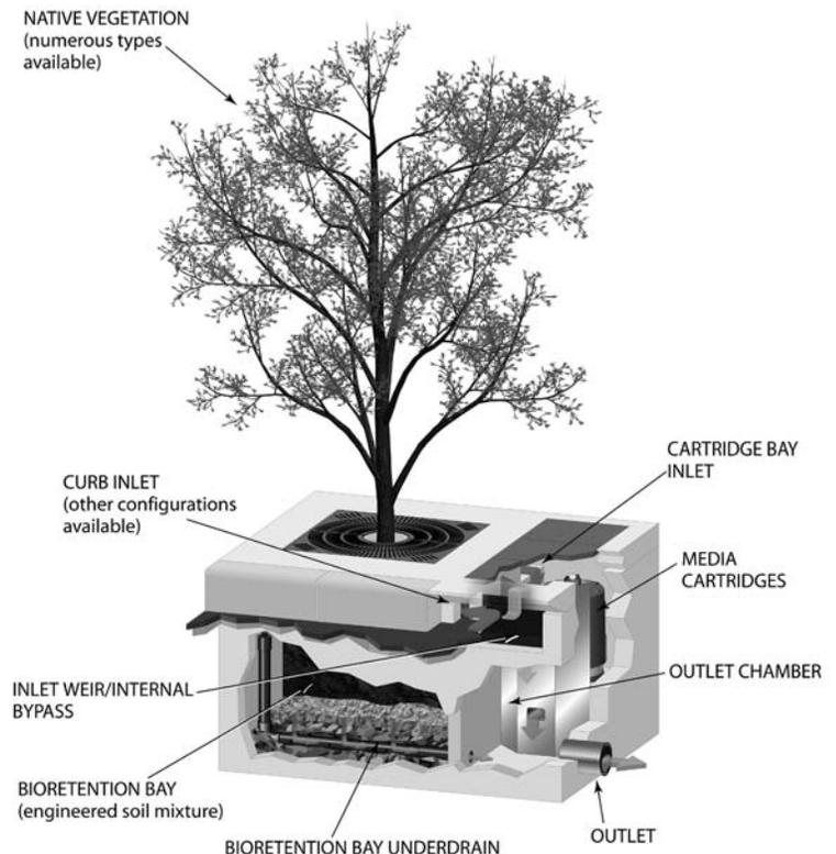
**Figure 1: Basic Operation & Components**
