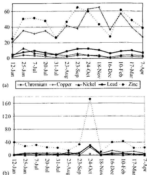
Fig. 2. Time series of (a) dry deposition flux in  $\mu\text{g}/\text{m}^2/\text{day}$  (MDL = 0.01) and (b) atmospheric concentration in  $\text{ng}/\text{m}^3$  (MDL = 0.03) based on sampling times/air volumes collected.
