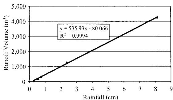
Fig. 1. Linear regression of rainfall vs. runoff measured in an urban Los Angeles catchment.
