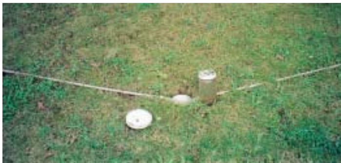
Figure 3. Tube-type lawn sampler (site 2).
