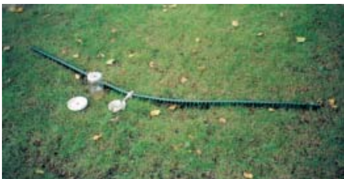
Figure 4. Edging-type lawn sampler (site 5).
