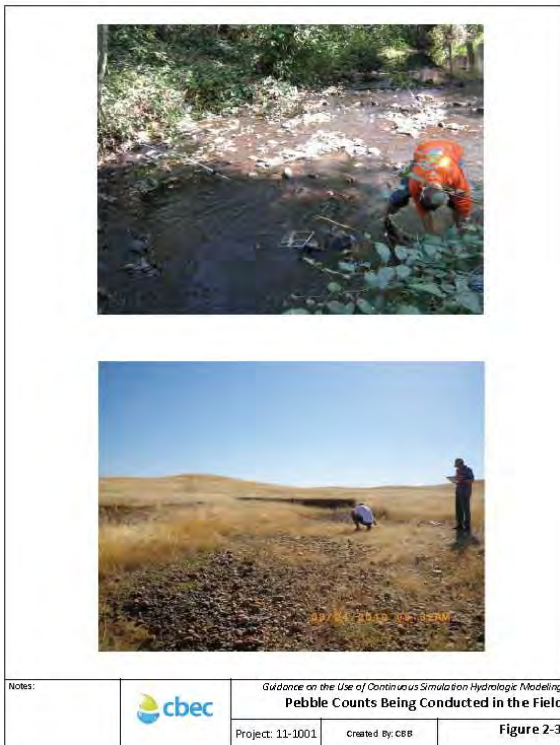
Figure 2-3. Pebble Counts Being Conducted in the Field
