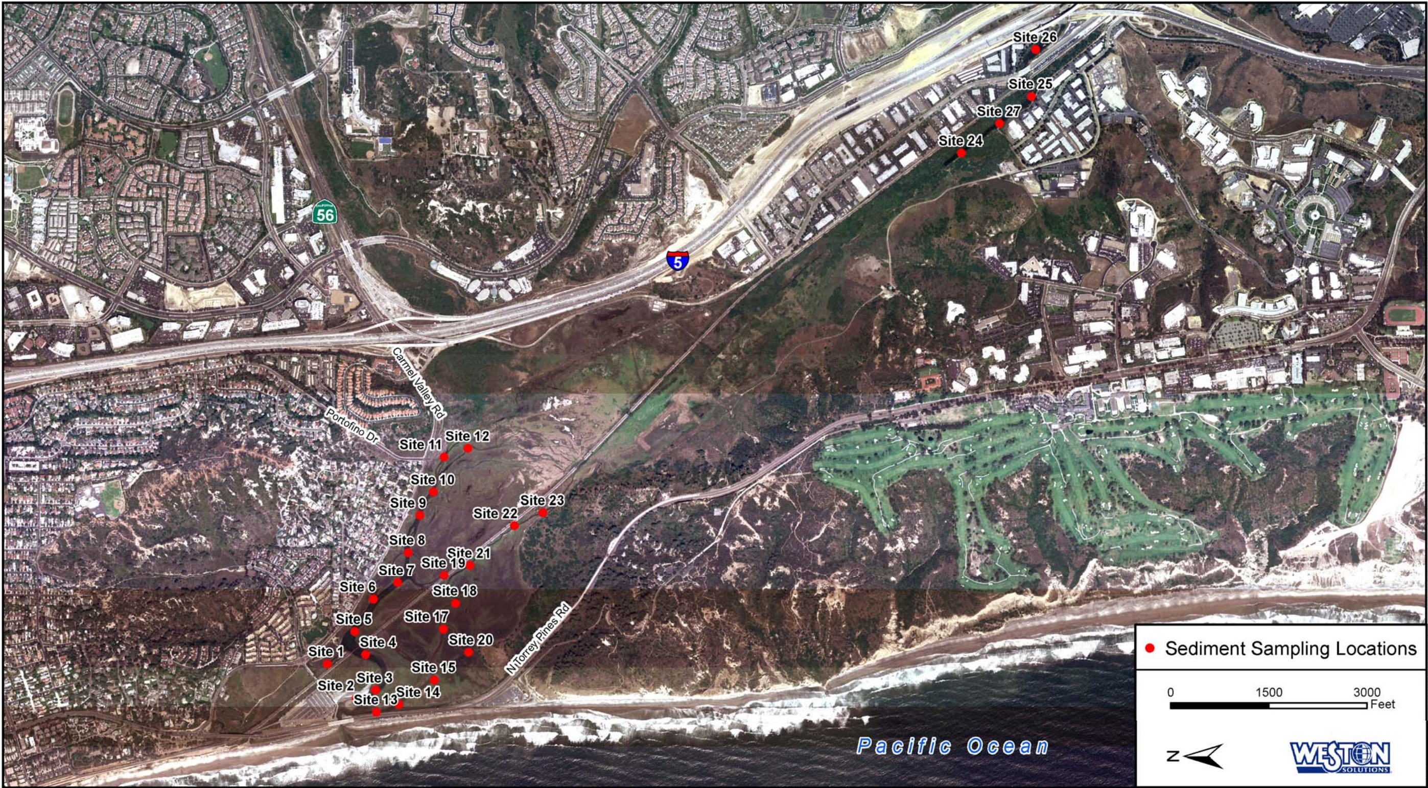
Figure 3-7. Post-Storm Sediment Sampling Locations in Los Peñasquitos Lagoon – February 11, 2008
