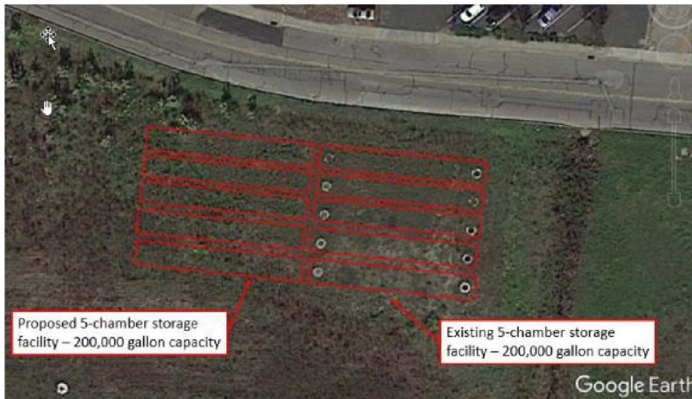
Figure 2. The project will expand existing storage capacity from 200,000 to 400,000 gallons.
